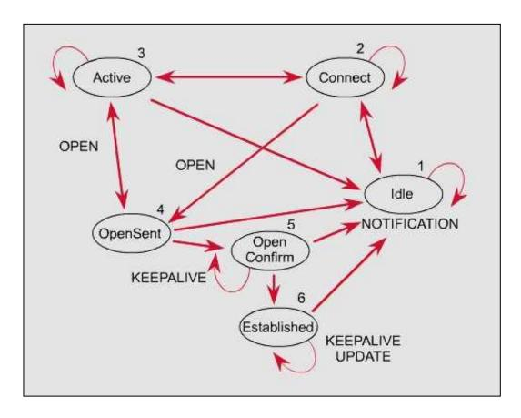
The BGP neighbor negotiation process proceeds through various states, or stages, which can be described in terms of a finite-state machine (FSM).
